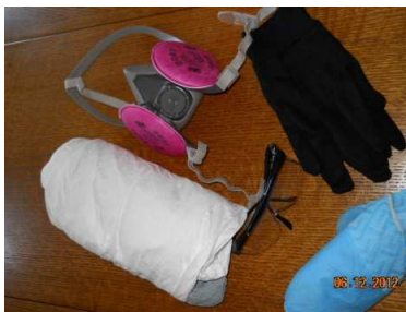
Examples of basic lead-safe renovation protective clothing. Depending on the job being performed, more protection might be needed.
